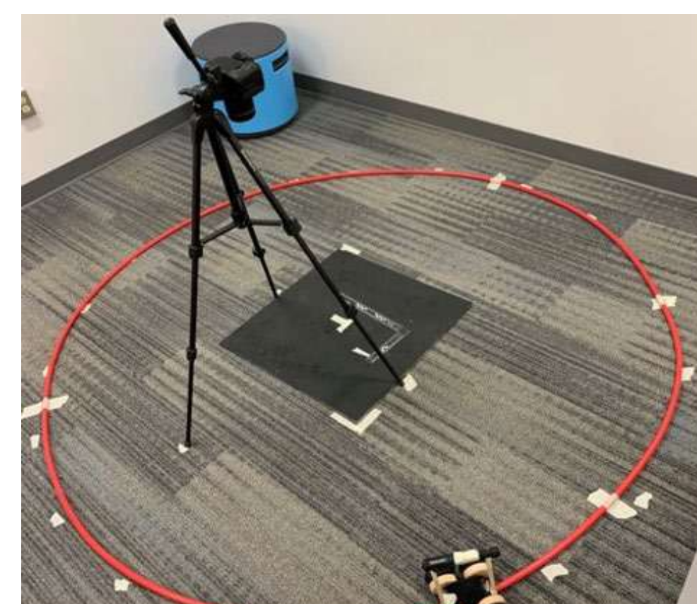
Figure 2 shows the setup used to capture images of gel lifts using the Rufus RC car for "light painting" to capture consistent images.
