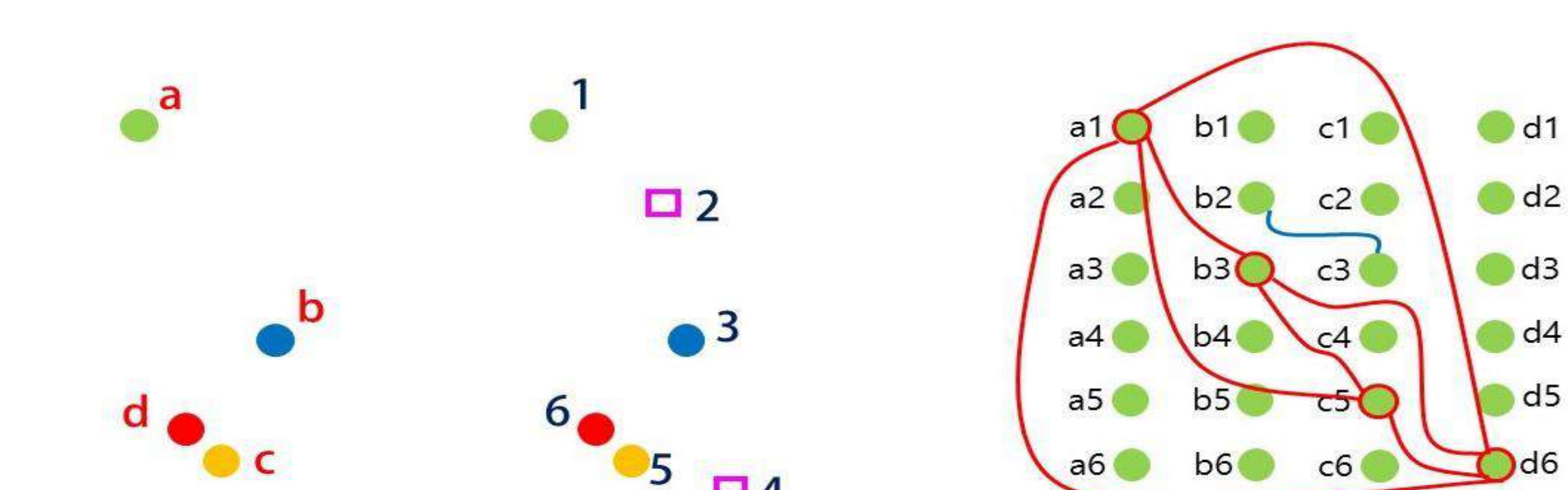
Figure (A) and (B) are example images. Image 1 has a set of points {a, b, c, d} and image 2 has a set of points {1, 2, 3, 4, 5, 6}. Figure (C) is application of the concept of maximum clique to find the correspondence between image 1 and image 2 is {(a,1), (b,3), (d,6), (c,5)}.
