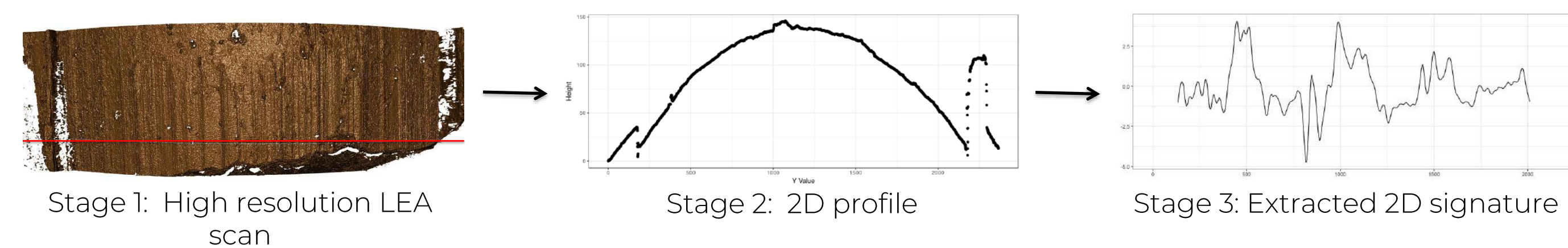
Figure 2: The process of extracting 2D data from a 3D scanning object, as Hare et. al. [1] describe.
