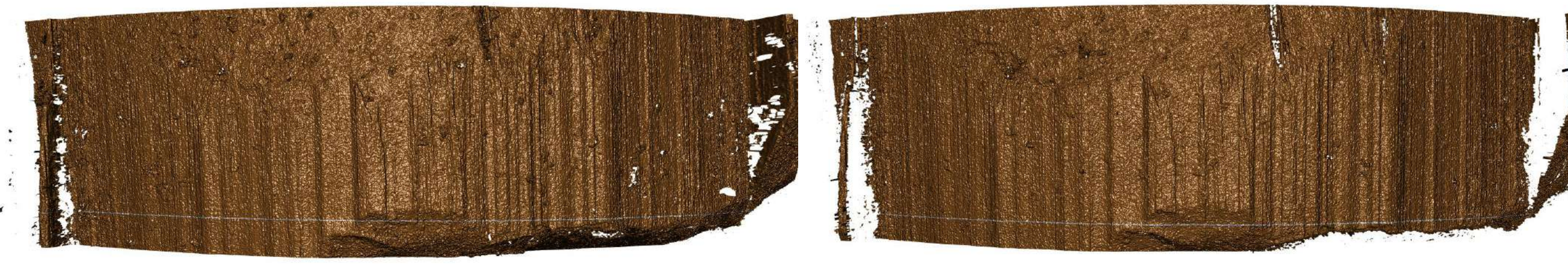
Figure 3: Two example LEA scans of the same barrel-land from the same bullet.
