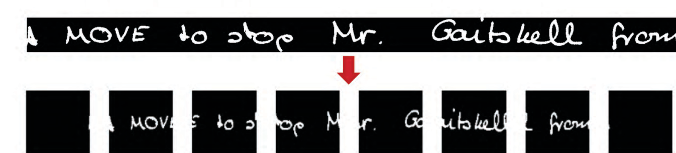
Figure 6: Segmented Images. Shows a line image being segmented into eight smaller images that contain parts of the line. Images that do not contain enough features, such as the first and last image in the partition are removed from the data set.
