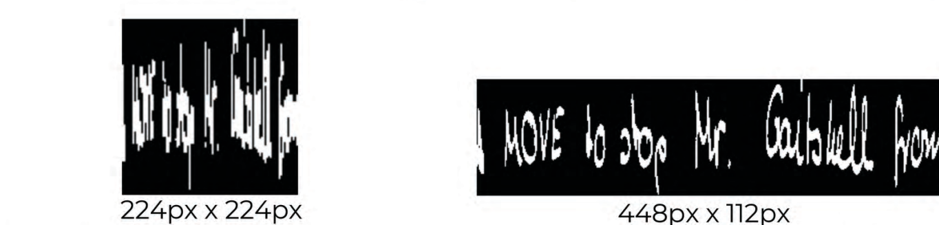
Figure 5: Resized Images. Comparing a square input to an input that has larger aspect ratio, the writing in the square image is more distorted but yields a denser image array of handwriting features.
