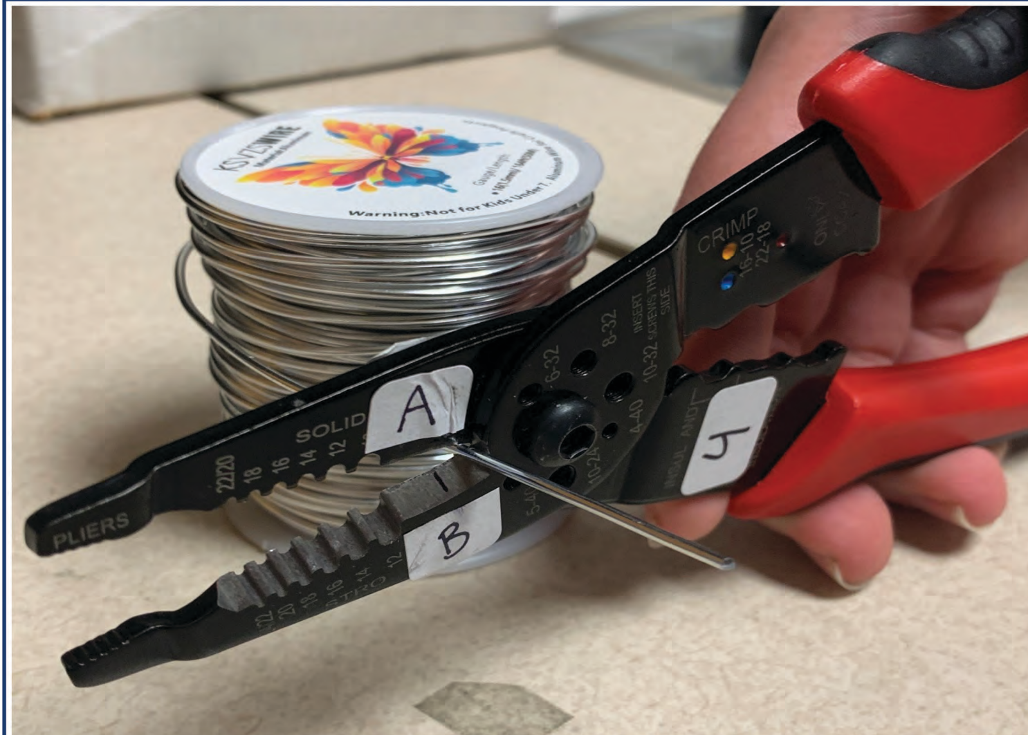
A Figure A shows an example of how we would get a test cut. For this image we are using pair 4 of our pliers making an AB test cut
