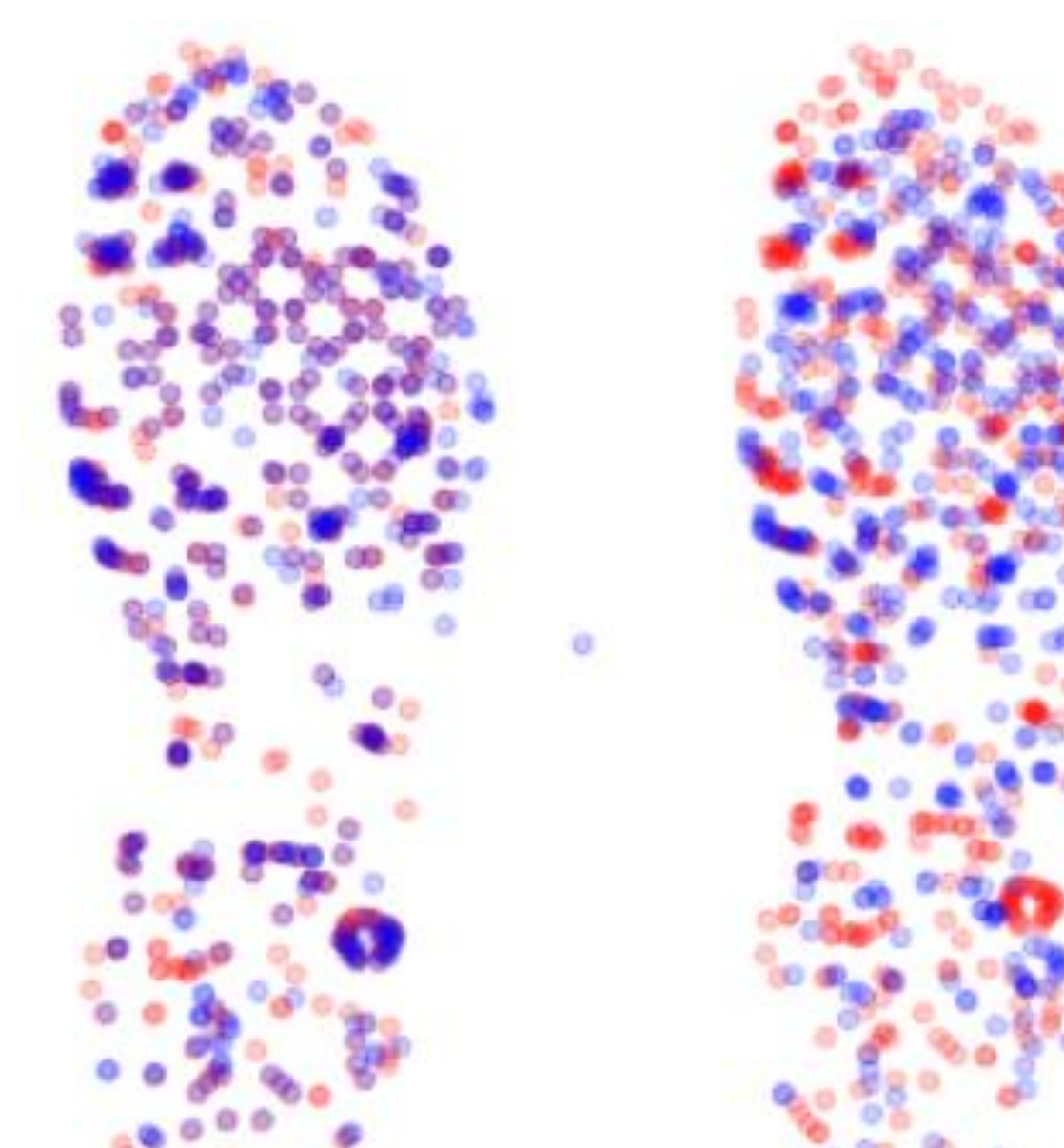
Alignment of shoe 4 (right side): SURF points from shoe 4 without extra weight is colored in red in both figures. Blue dots on the left, and right figures indicate the same shoe without extra weight, and with extra 55lb, respectively.
