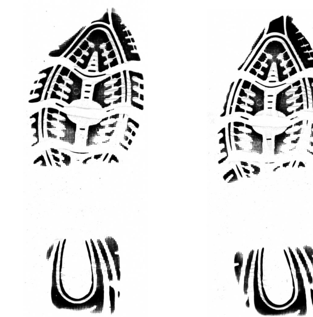
Impression of shoe 1 (left side) using EverOS: the image on the right was by a person, and the image on the left was with added 55lb to the person.
